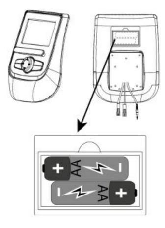
The console is equipped with 2 AA batteries at the rear of the console.
