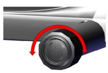
Adjust the foot caps by twisting them in either direction to avoid rocking movements of the workout equipment.
