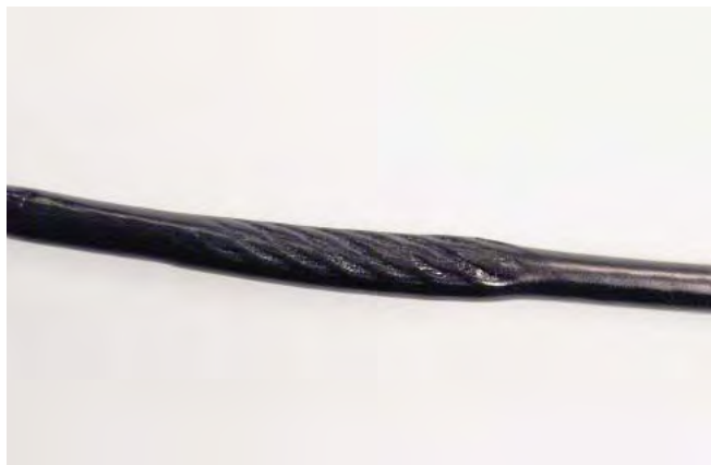
"NECKING", STRECHED CABLE COVERING
