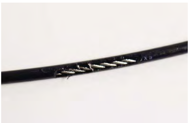
A TEAR IN THE CABLE COVER
