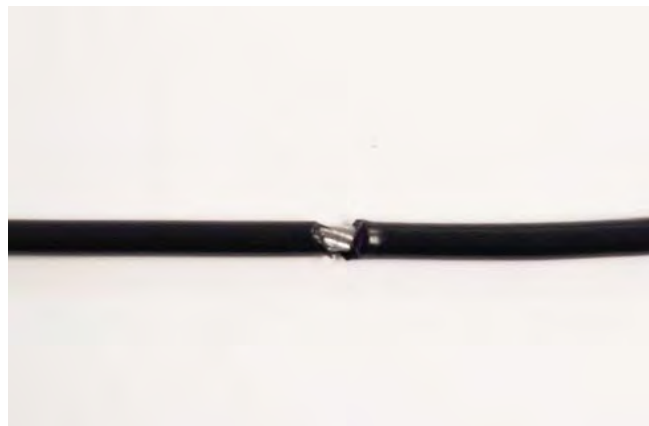
A CRACK IN THE CABLE COVER
